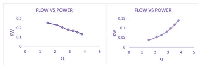
Figure 9. Flow Vs Power (a) Throttling (b) VFD
